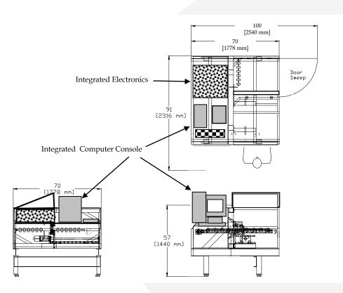
Figure 1: AS-150-MAX Overall Machine Dimensions
