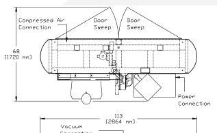
Figure 1: AS-200-JM Overall Machine Dimensions
