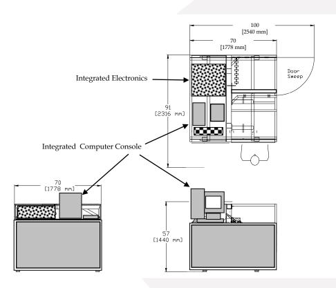
Figure 1: AS-100-MAX Overall Machine Dimensions
